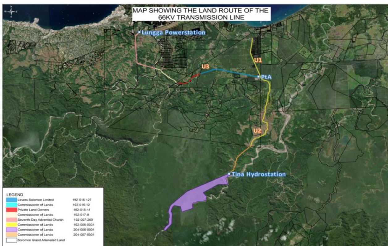
Figure A1-5, below is the SIEA's 50m corridor route of the 66kV Transmission Line, from the Hydropower facility to Lungga Diesel Power Station. The Project will finance only the line from Tina Hydro-Station to Lungga Power Station (route sections U2+U3 = 22km). SIG registered route sections = U1+U2.
